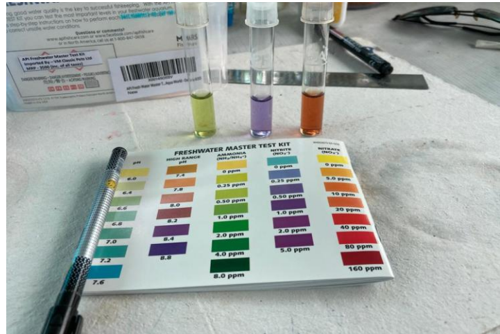
Ammonia, Nitrite, Nitrate test (API kit)
